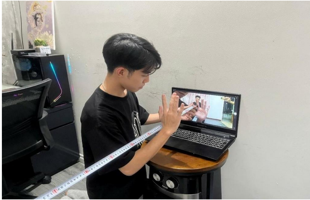
Figure 11: Calibration Physical Setup for Measuring Distance vs. Pixel Spacing
